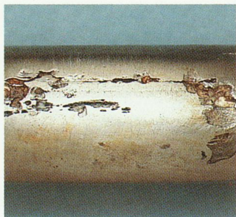
Barnacle build-up on this swim platform led to crevice corrosion.
